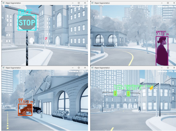
Fig. 4: Key object types considered in the resilience design: stop sign, pedestrian, vehicle ahead, and traffic light.
